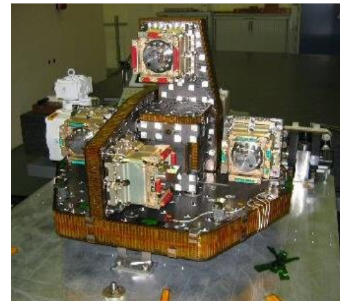
GOCE gradiometer is a set of electrostatic servo-controlled accelerometers
