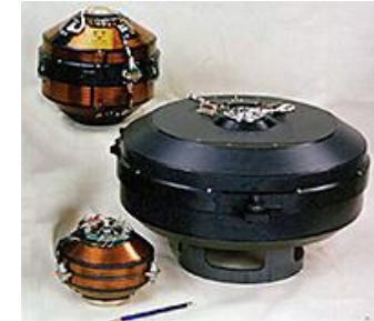
Lockheed Martin gradiometer consists of two opposing pairs of accelerometers arranged on a spinning disc
