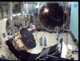
On station thermal tests
