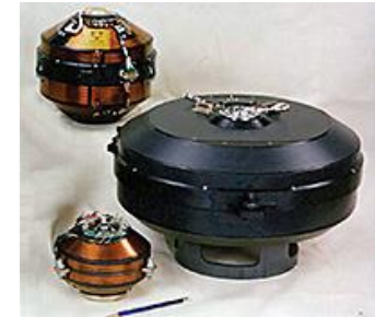
Lockheed Martin gradiometer consist of two opposing pairs of accelerometers arranged on a spinning disc
