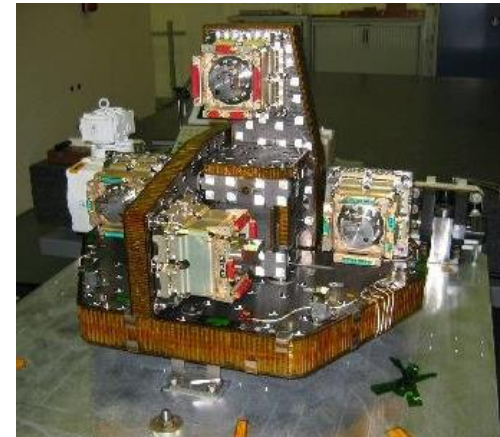
GOCE gradiometer is a set of electrostatic servo-controlled accelerometers
