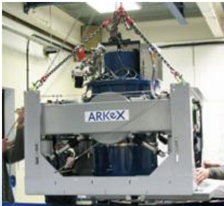
ARKeX gradiometer uses super conductivity for levitation of the proof masses and for the inherent stability
